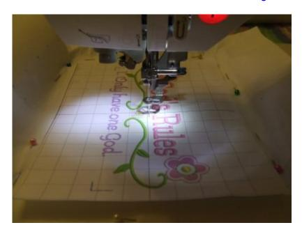
Once your needle is positioned directly over the marked center on the template, remove the template and begin your first stitchout. Notice the 2 removeable blue lines that are stitched out last that make rehooping this design a snap!
